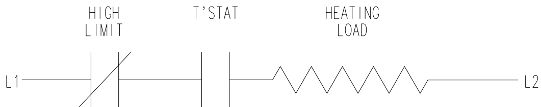
FIGURE 5. Wiring Diagram - XP Convection Heater
