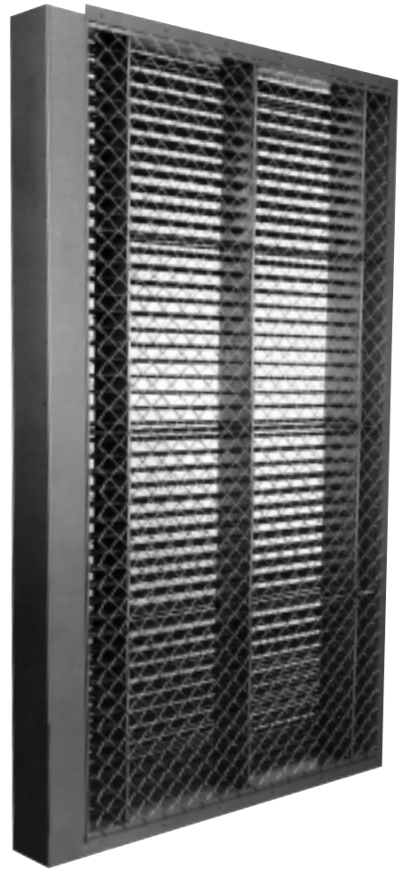
MINE VENT DUCT HEATER 600V 3Ø 320KW 21500 SCFM 9 FT x 5 FT
