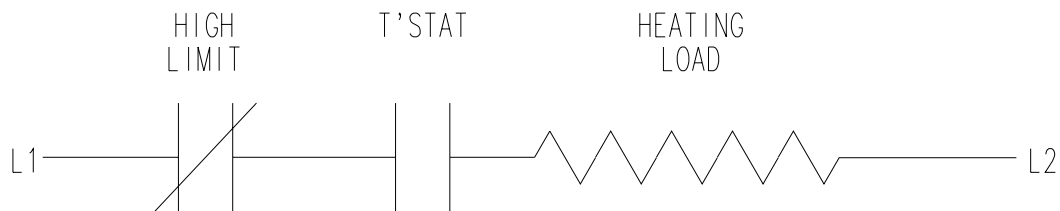
FIGURE 5. Wiring Diagram - XP Convection Heater
